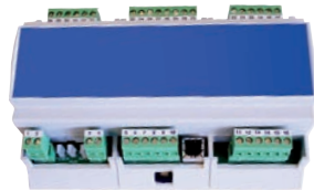
Signal calibration box
